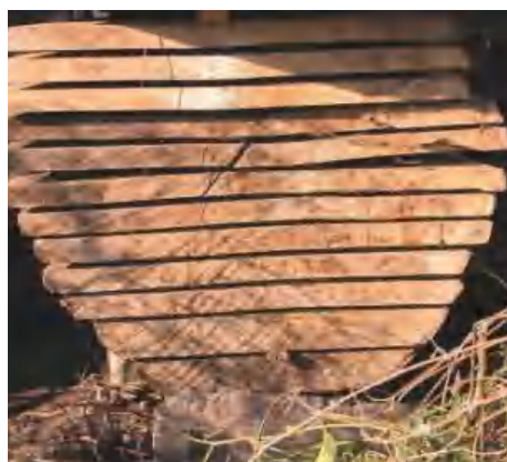
▲ Pic.7 When the log has been sliced the boards are kept in sequence
